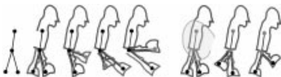
Figure 2: To create a simple walking figure, the user first creates the skeleton and fleshes it out. He then drags the feet to make the character walk. Next, he selects the control structure of the upper body and records its motion.
