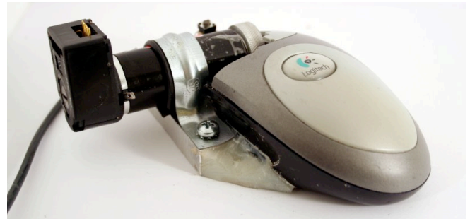
Figure 1. Mouse with haptic mousewheel
