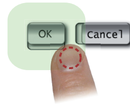
Figure 3: The slider thumb of the OK button can be moved by any touch within the highlighted green area. The Cancel button track is orthogonal to the OK button to avoid accidental activation.
